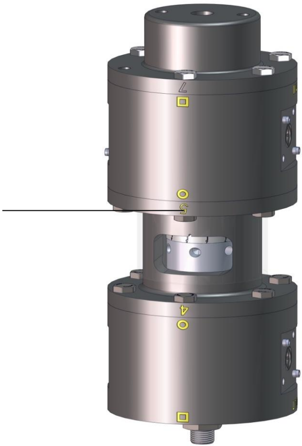
Power Module Assembly with Pilot Bottom Flange Installed (QTY 1)
